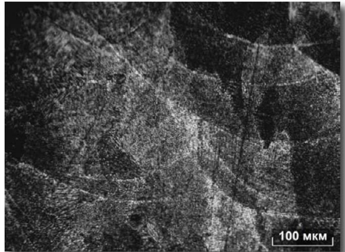
Pictures of microstructure of samples from austenitic corrosion-resistant steel 12X18H10T manufactured at MeltMaster<sup>3D</sup>-550
