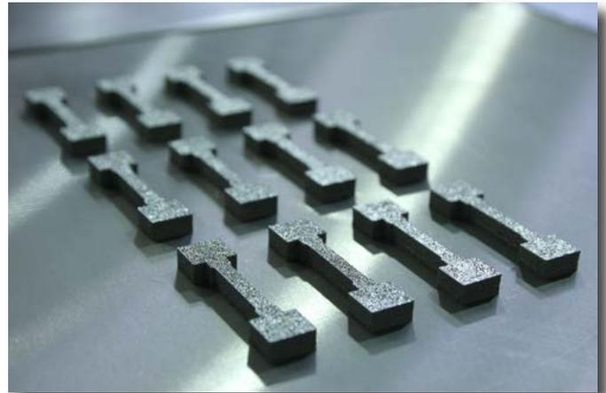
Samples fabricated at MeltMaster<sup>3D</sup>-550
